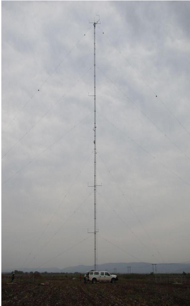
**Figure 2:** Wind turbine data collection station used at the WM12 and the WM13 sites [6]
