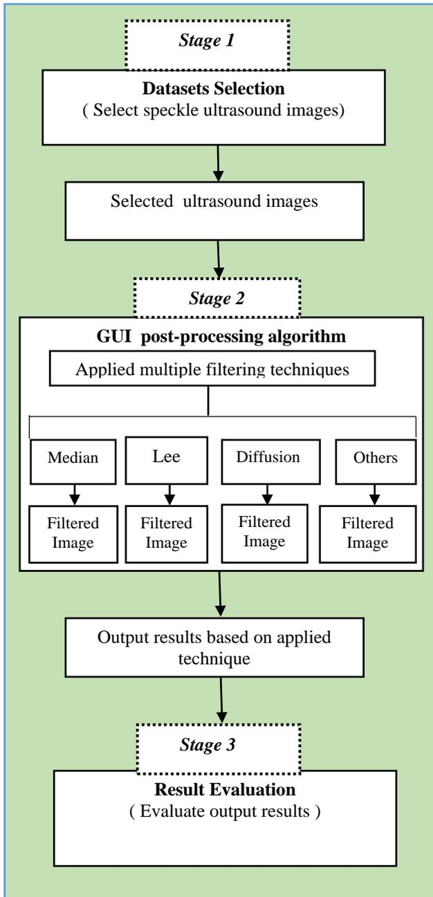
**Figure 1:** Structure and block diagram of developed speckle noises reduction on an ultrasound image
