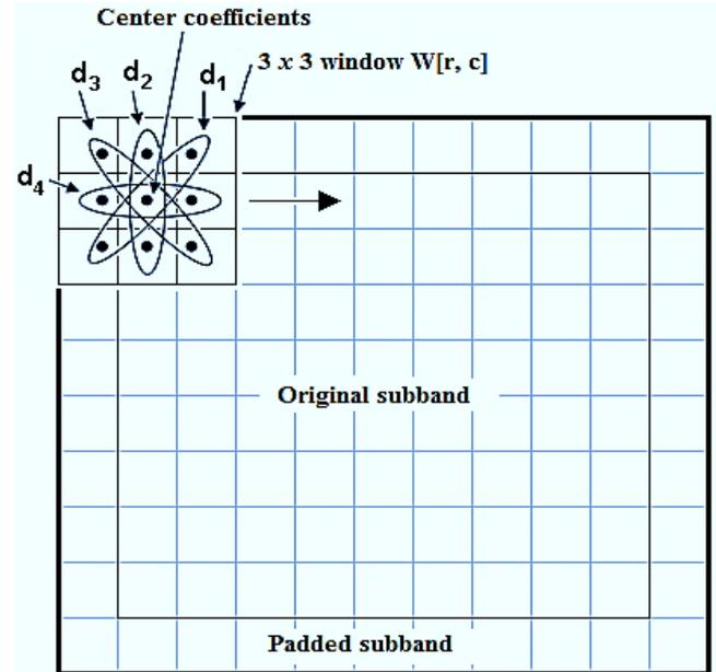
Figure 1: A 3 x 3 filter window on a particular sub-band
