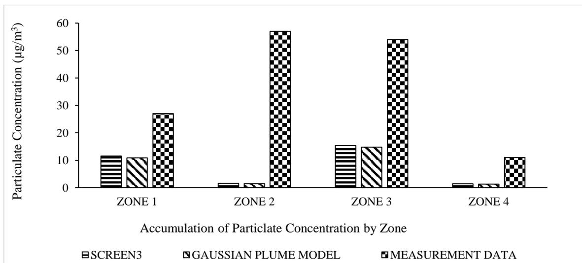
**Figure 6.** Comparison between particulate accumulation concentration by using the SCREEN3, Gaussian Plume Model, and measurement data
