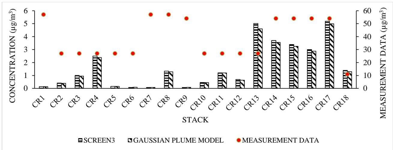
**Figure 5.** Comparison between simulated particulate maximum concentration by the SCREEN3 Model and Gaussian Plume Model for 18 stacks
