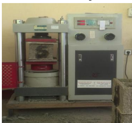
Figure 2. Compressive strength test for HCB
