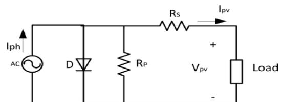
Figure 2: Equivalent diagram of PV cell
