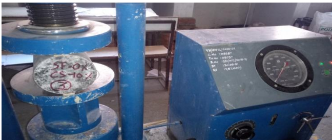
Fig.9 Split Tensile Strength Testing
