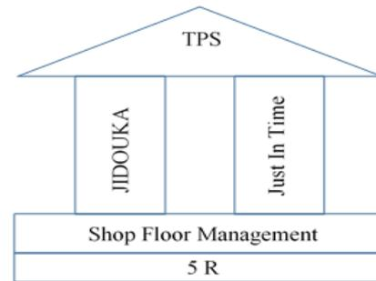
Figure 3. Foundation and Pillar of manufacture production svstem
