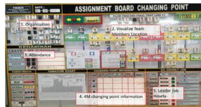
Figure 8. Changing point Control board at shop floor
