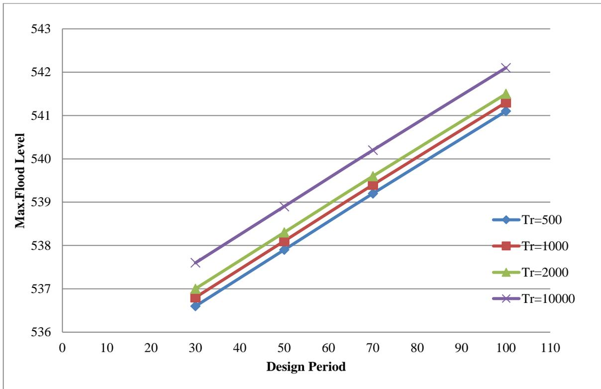
**Figure (7)** Maximum Flood Levels for different Return and Design Periods
