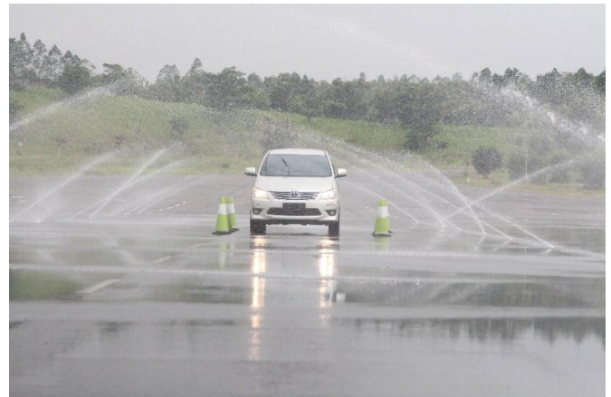
Figure 1. Wet Braking Test Condition
