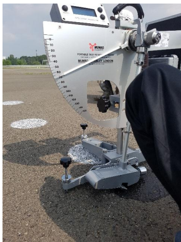
Figure 2. Test the roughness of asphalt with BPT
