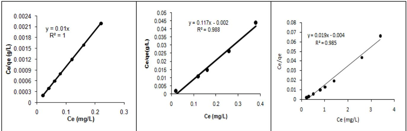
Fig.6 : Langmuir isotherm model for the three dyes
