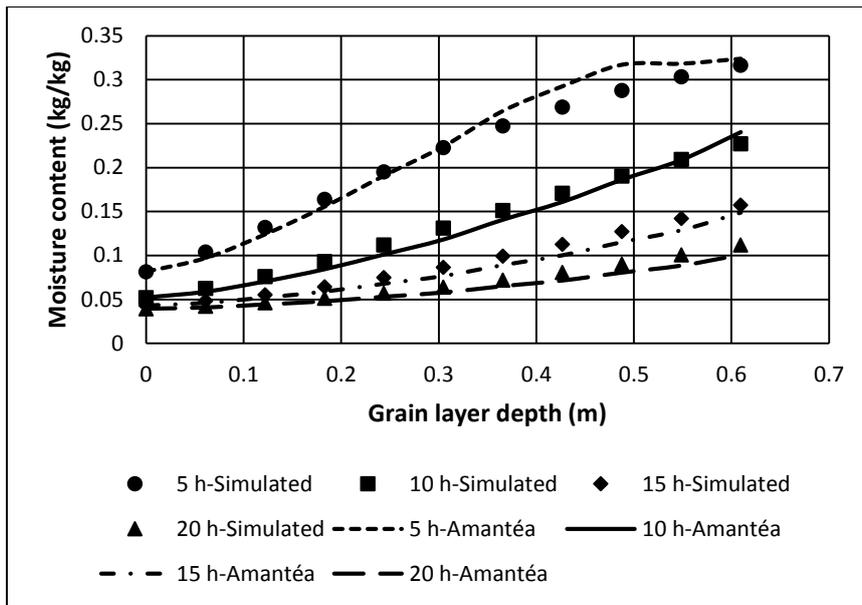
**Figure 51.** Moisture content of the product X grain layer depth.
