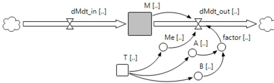
**Figure 5.** Product moisture content simplified flux diagram.
