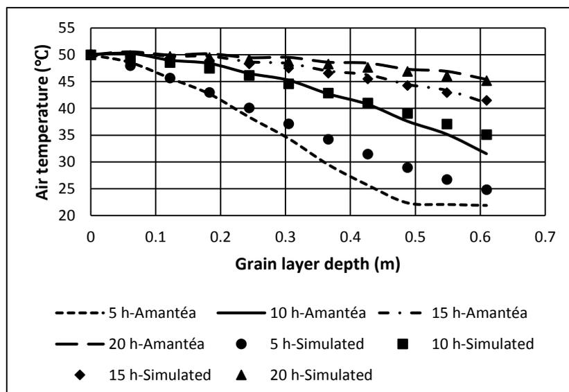
**Figure 7.** Air temperature X grain layer depth.
