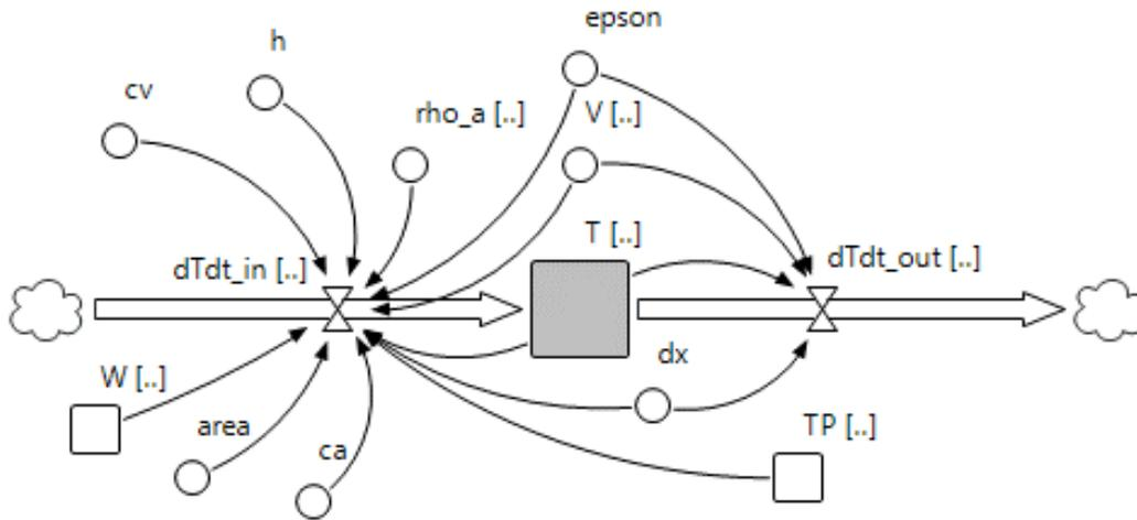
Figure 4. Air temperature simplified flux diagram.
