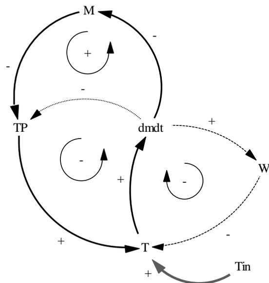
Figure 2. Causal diagram of deep layer drying.
