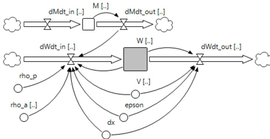
**Figure 6.** Simplified air humidity ratio flux diagram.
