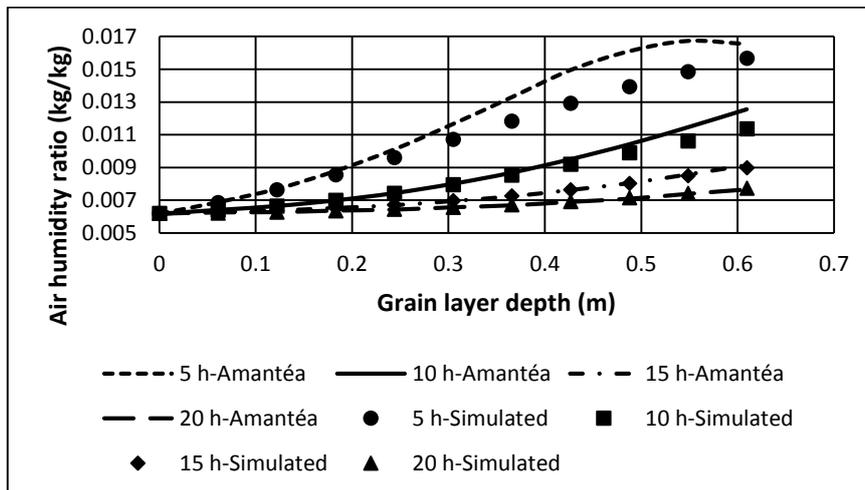
**Figure 126.** Humidity ratio X grain layer depth.
