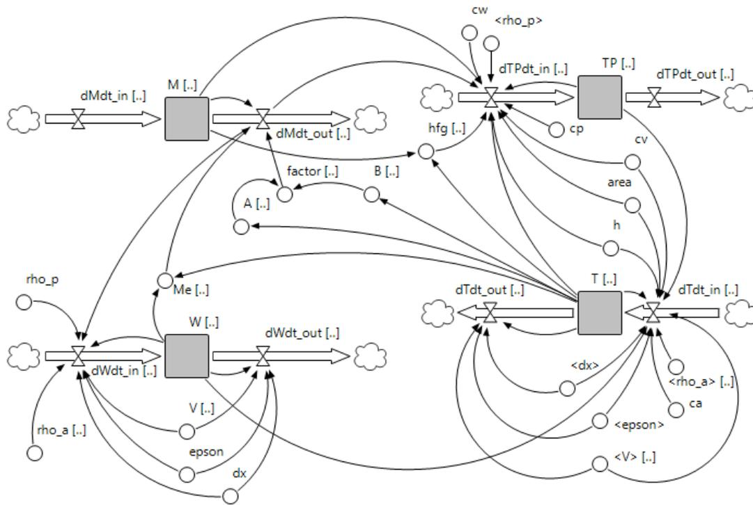
Figure 9. Complete flux diagram of the deep layer grain drying model.
