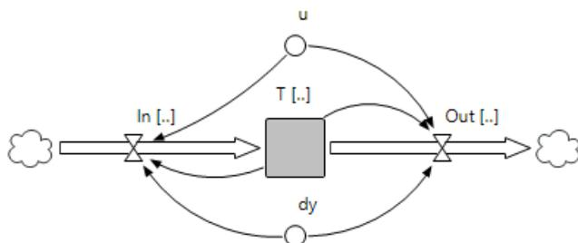
**Figure 3.** Pure convection equation representation in the Anylogic software.
