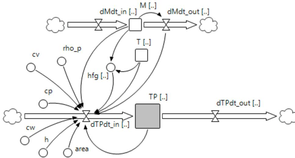
**Figure 7.** Product temperature simplified flux diagram.
