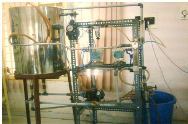
Fig. 2 Photographic view of the integrating tank experimental setup.
