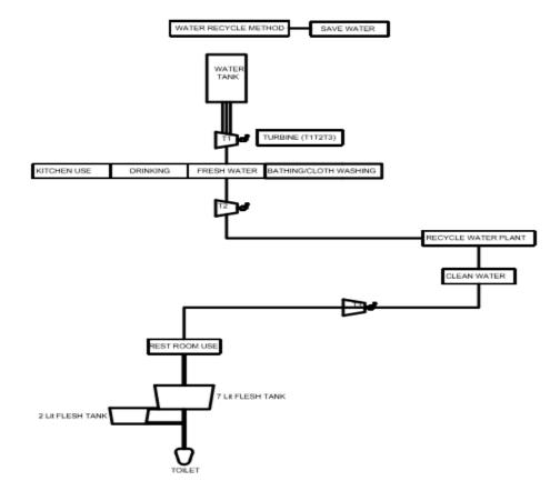
Figure 1. Water re-cycle layout.
