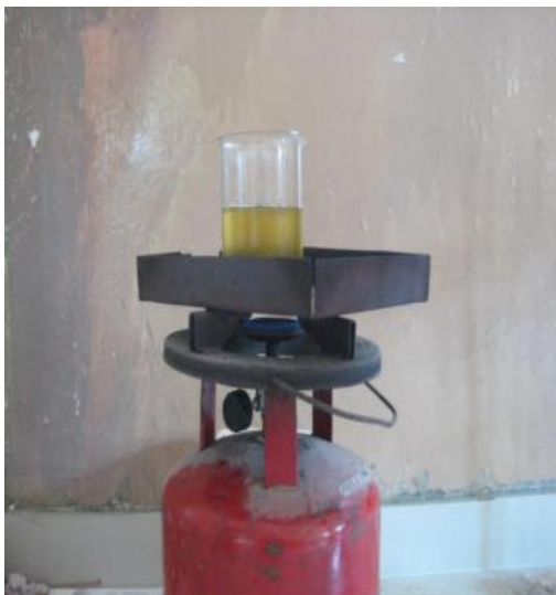
Fig 6: Heating of collected methyl ester
