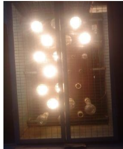
Fig. 2: Engine test rig subjected to load (each bulb shown is of 500W).
