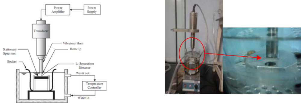
Fig. 7: Cavitation test setup.
