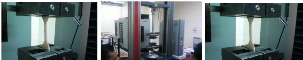
Fig. 4: Universal Testing Machine & Grips of the testing machine (Zwick / Zwick / Roell Z010 )
