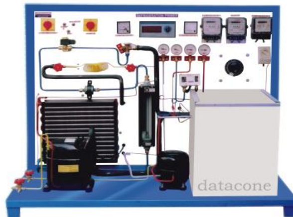
Fig. 1: Experimental Setup of the refrigeration test rig
