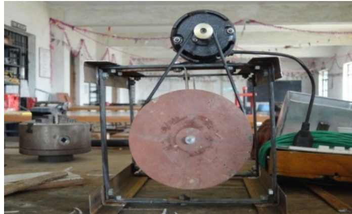
Fig. 2. The pulley and belt system attached with the motor
