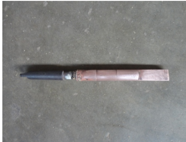
Fig. 4. Workpiece fixture with free-form job fabricated from copper alloy
