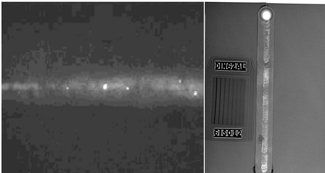
Fig. 5 Irregularly shaped lower density spots randomly located in the weld image
