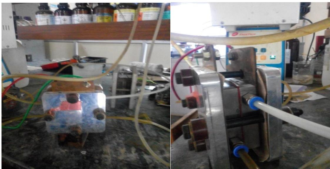
**Figure 2:** Proton Exchange Membrane (PEM) Single Cell
