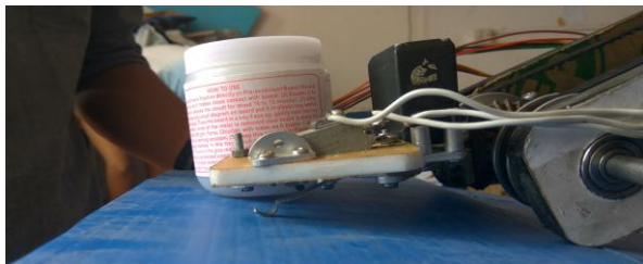
Fig. 6 Determining the platform existence for placing object
