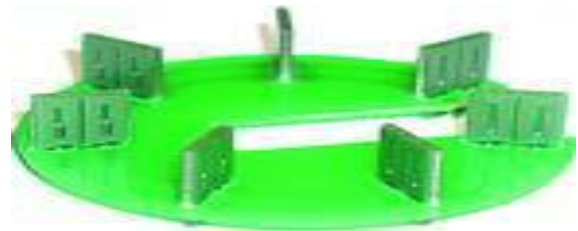
Fig. 2. PCB based Rogowski Coil [12]
