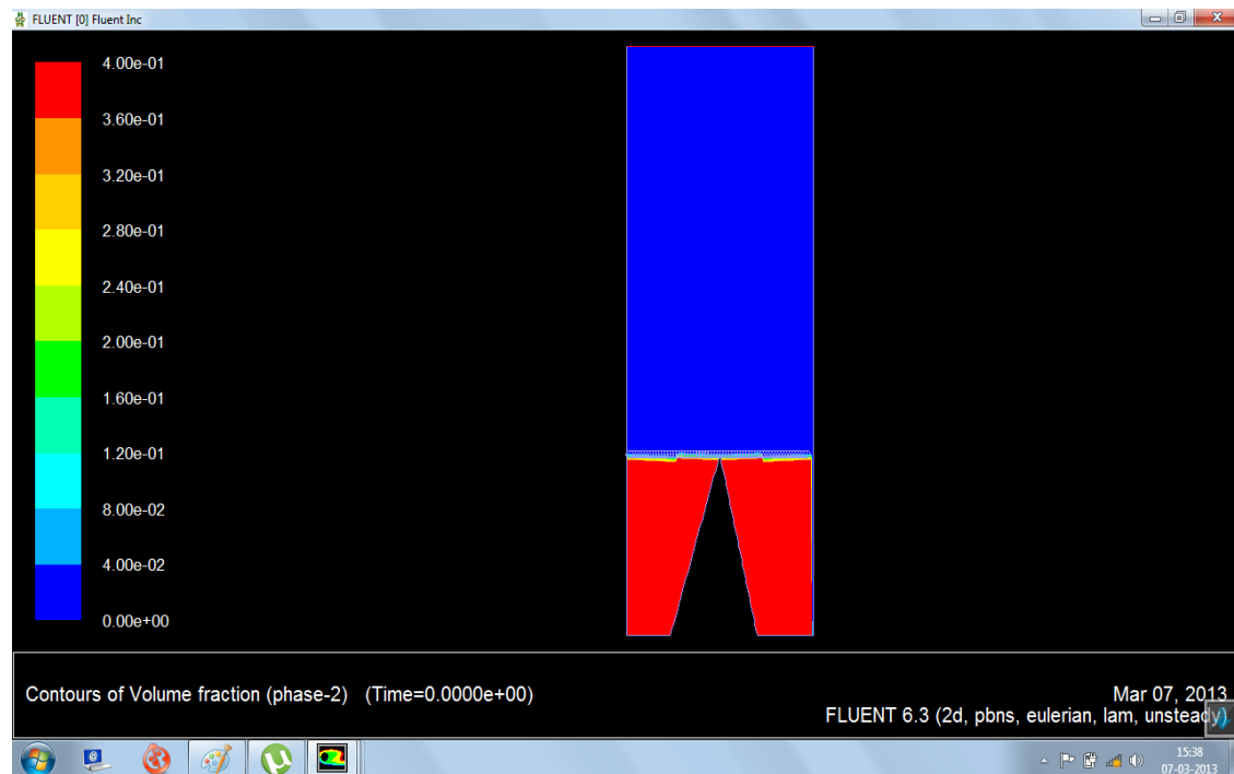
Fig.10. Initial condition of the fluid bed U < U_{mf}
