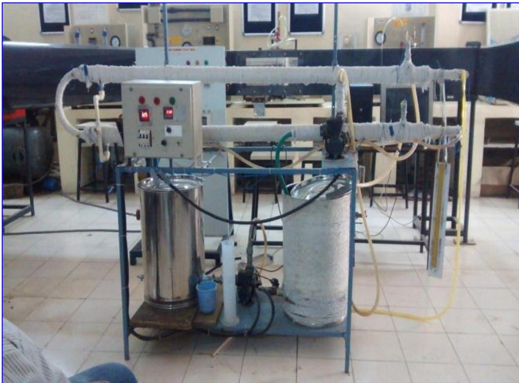
**Fig. 1** Experimental set up of double pipe U-bend heat exchanger
