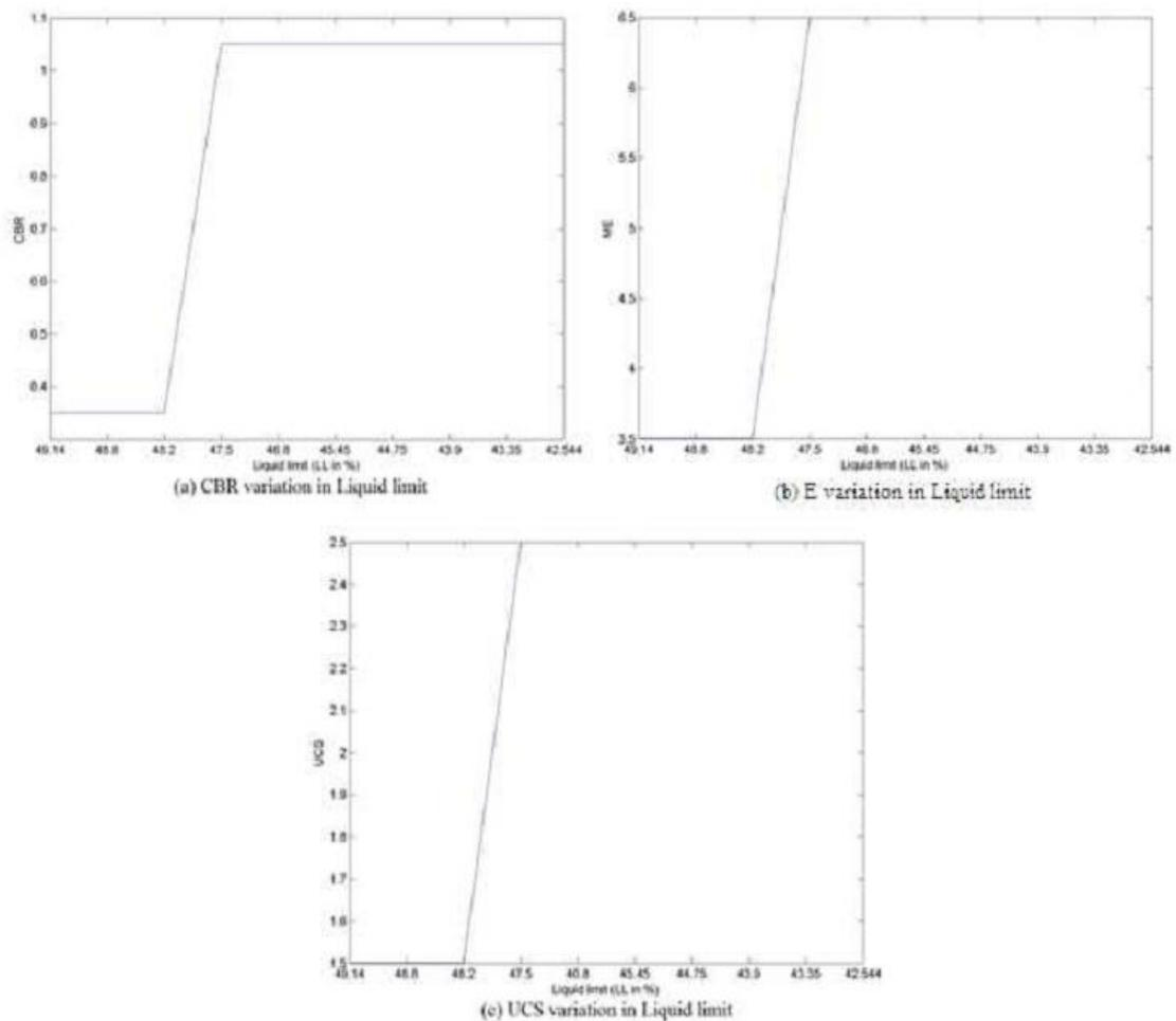
**Fig.1:** Liquid limit Vs outputs
