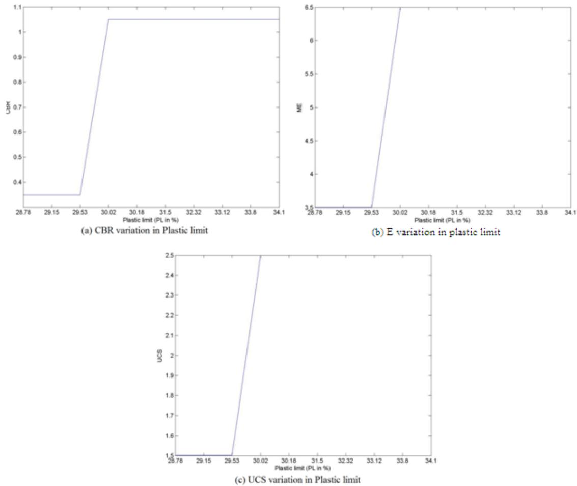
**Fig.2:** Plastic limit Vs output
