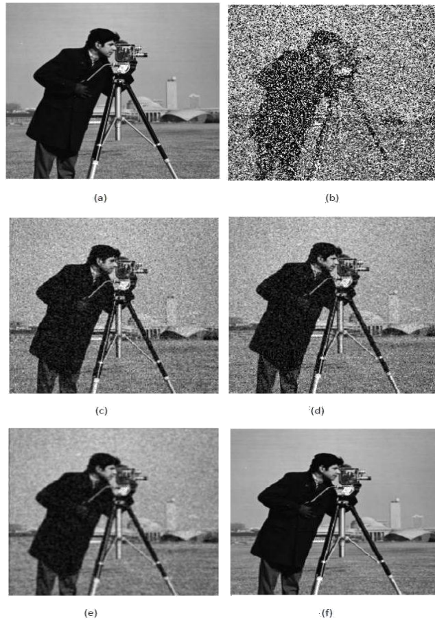
Figure 2: Simulation results for 60% corrupted 'cameraman' image (a)original image (b) noisy image (c) DWMF (d)EDRIN (e) RDRIN (f) Proposed method
