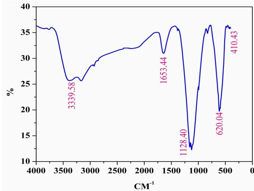
**Figure 2:** IR spectrum of  $\text{Ni}_{0.6}\text{Co}_{0.2}\text{Zn}_{0.2}\text{Fe}_{2-y}\text{La}_y\text{O}_4$  ( $y=0.050$ ).
