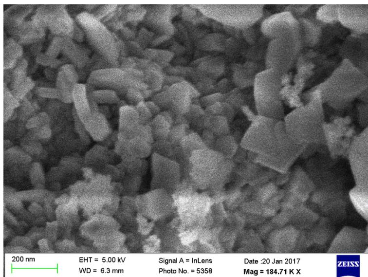
**Figure 3:** SEM image of Ni<sub>0.6</sub>Co<sub>0.2</sub>Zn<sub>0.2</sub>Fe<sub>2-y</sub>La<sub>y</sub>O<sub>4</sub> (y=0.05).
