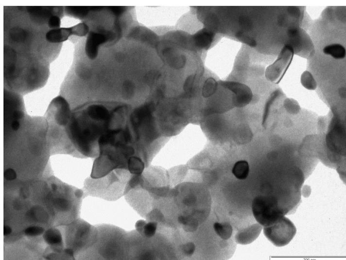
**Figure 4:** TEM image of Ni<sub>0.6</sub>Co<sub>0.2</sub>Zn<sub>0.2</sub>Fe<sub>2-y</sub>La<sub>y</sub>O<sub>4</sub> (y=0.05).
