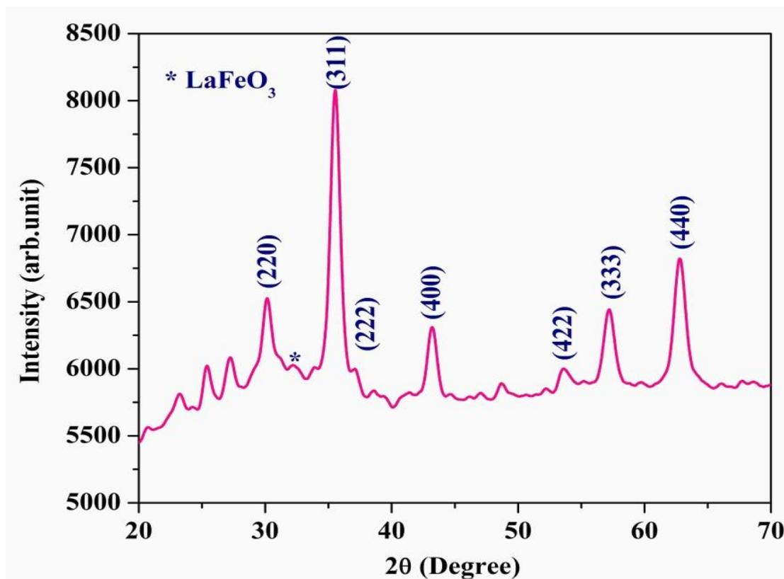
**Figure 1:** XRD spectrum of  $\text{Ni}_{0.6}\text{Co}_{0.2}\text{Zn}_{0.2}\text{Fe}_{2-y}\text{La}_y\text{O}_4$  ( $y=0.050$ ).
