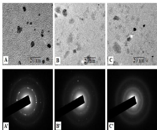
**Fig. 3** High-resolution (HR) TEM images, SAED patterns of ZnTe:Cu QDs.
