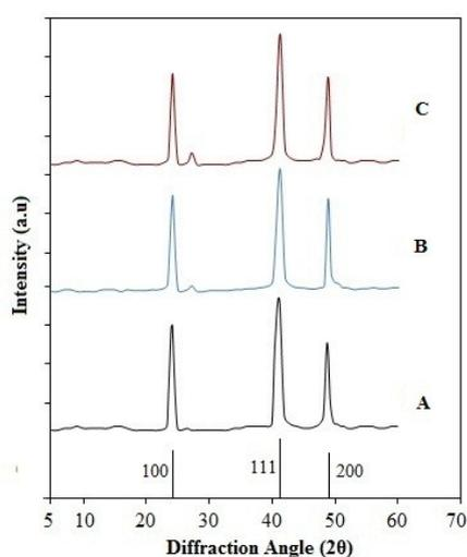
**Fig. 1** X-ray diffraction (XRD) patterns of ZnTe:Cu samples.
