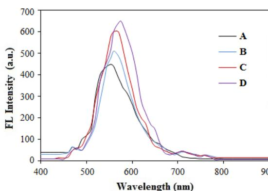
**Fig. 7** Fluorescence spectra of the ZnTe:Cu QDs.
