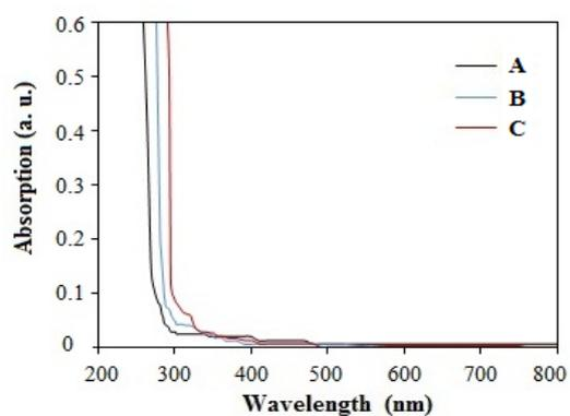
**Fig. 5** Optical absorption spectra of ZnTe:Cu QDs.
