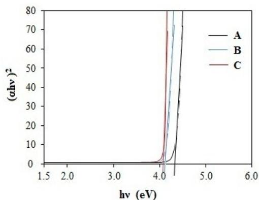
**Fig. 6** Band gap energy spectra of ZnTe:Cu
