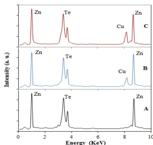
**Fig. 2** EDAX patterns of ZnTe:Cu samples.
