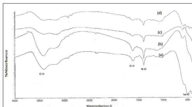
**Fig. 4.** FTIR pattern of SnO Nanoparticles Synthesized at 150°C for (a) 1hr (b) 2 hrs (c) 3hrs (d) 4hrs
