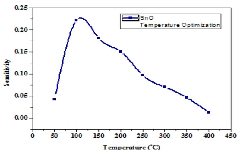
**Fig.11.** Gas sensing response of nano SnO
