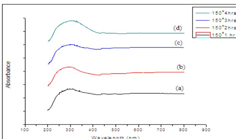
**Fig.6.** UV-DRS Spectra of SnO Nanoparticles Synthesized at 150°C for (a) 1hr (b) 2 hrs (c) 3hrs (d) 4hrs
