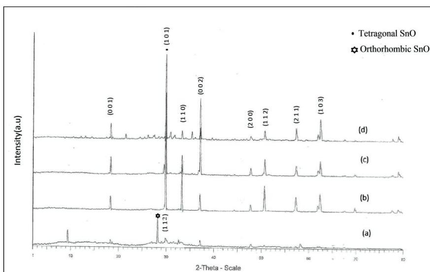
**Fig 1.** XRD pattern of SnO nanoparticles synthesize for 4hrs at (a) 120°C (b) 150°C (c) 180°C & (d) 200°C
