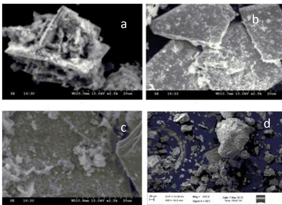
**Fig.7.** SEM micrographs of the SnO nanoparticles synthesized at (a) 120°C, (b) 150°C, (c) 180°C & (d) 200°C
