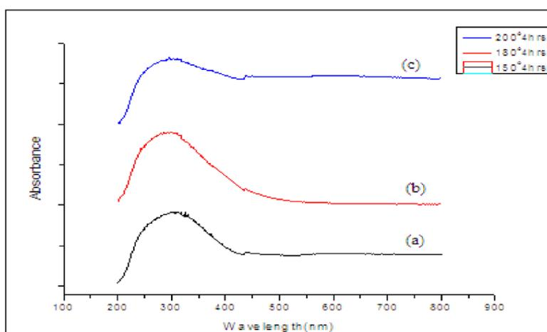
**Fig.5.** UV-DRS Spectra of SnO Nanoparticles Synthesized for 4 hrs at (a) 120°C (b) 150°C (c) 180°C (d) 200°C
