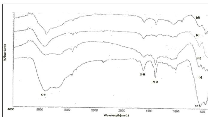
**Fig.3.** FTIR Spectra of SnO Nanoparticles Synthesized for 4 hrs at (a) 120°C (b) 150°C (c) 180°C (d) 200°C
