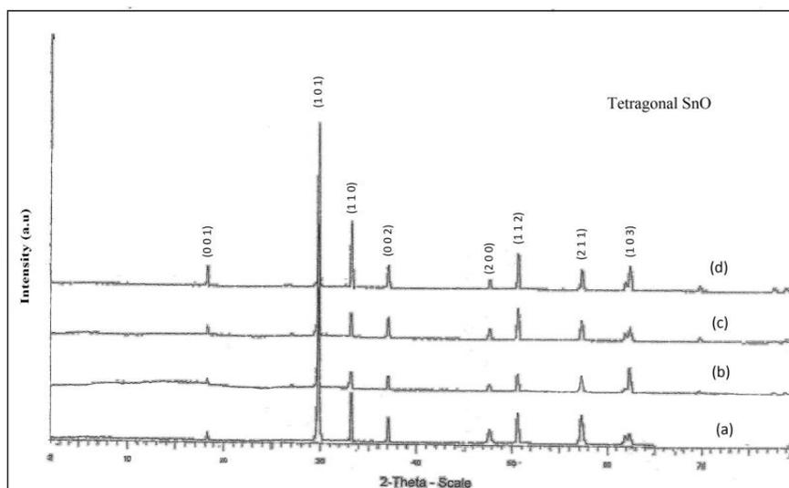
**Fig. 2.** XRD pattern of SnO nanoparticles synthesized at 150°C for (a) 1hr (b) 2hrs (c) 3hrs & (d) 4hrs
