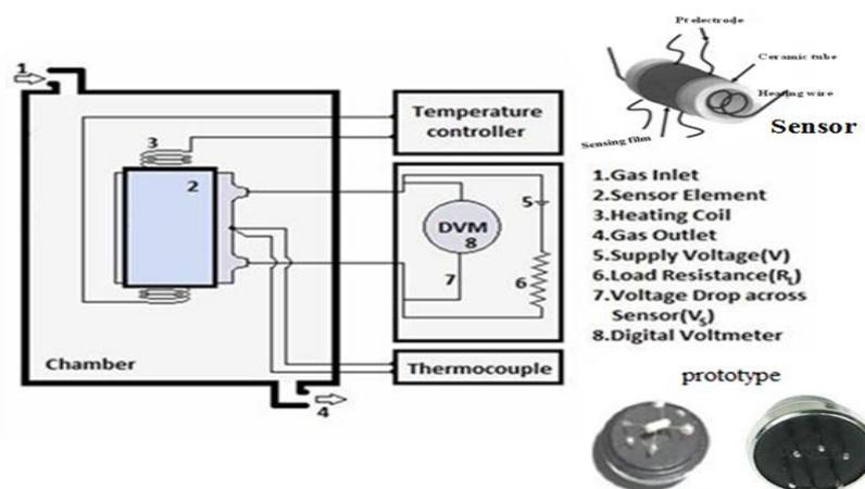
**Fig.10** Schematic representation of gas sensor Measurement setup
