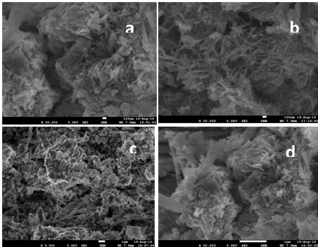
**Fig.8.** SEM micrographs of the SnO nanoparticles synthesized at 150°C for (a) 1hr, (b) 2hrs, (c) 3hrs & (d) 4hrs
