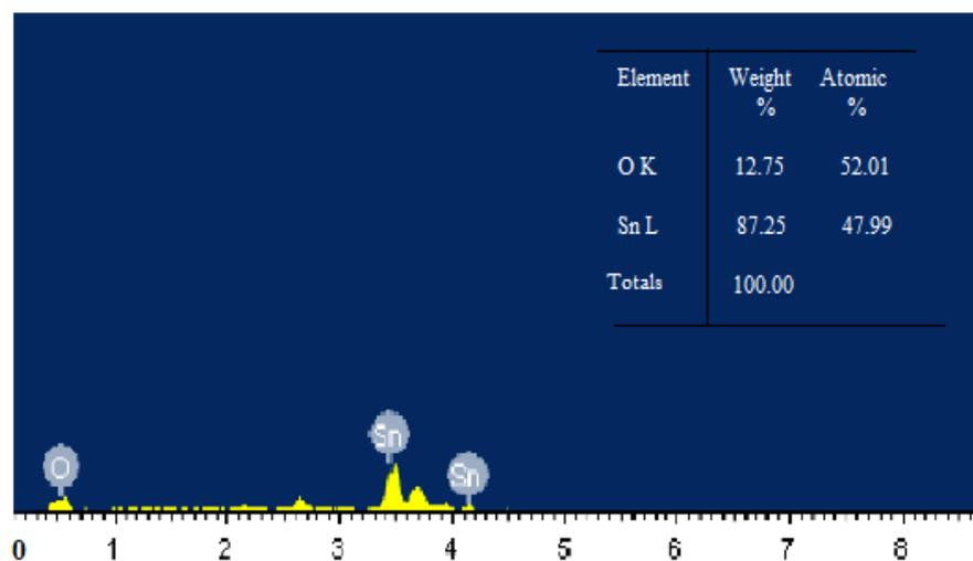
**Fig.9.** EDAX spectrum of SnO nanoparticles
