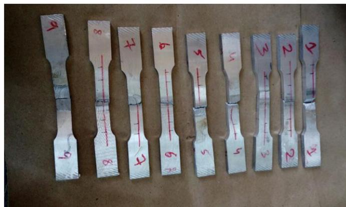
**Figure 7: Tensile test specimen after testing**
