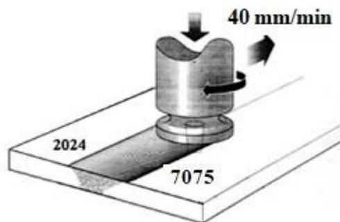
**Figure 1: FSW process of 2024-7075 aluminium alloys**
