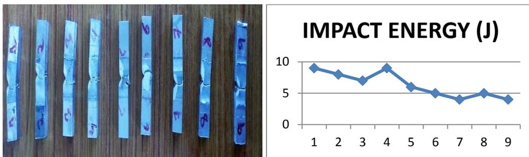
**Figure 8: specimen after conducting impact test**
