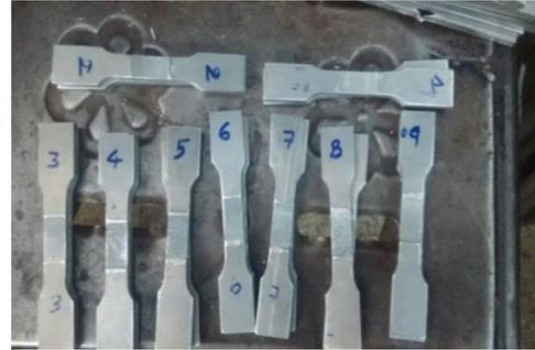
**Figure 3: Tensile test specimen cutting nomenclature**
