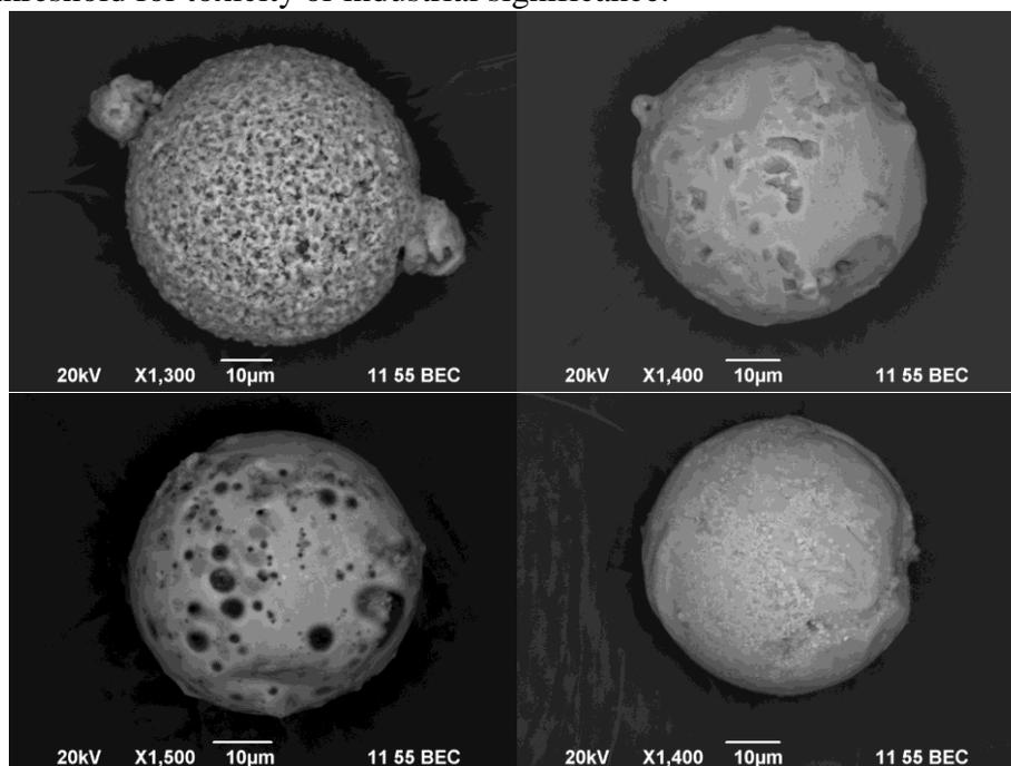
**Fig. 1** – Micro-spheres from ASW photographed under a scanning electron microscope
