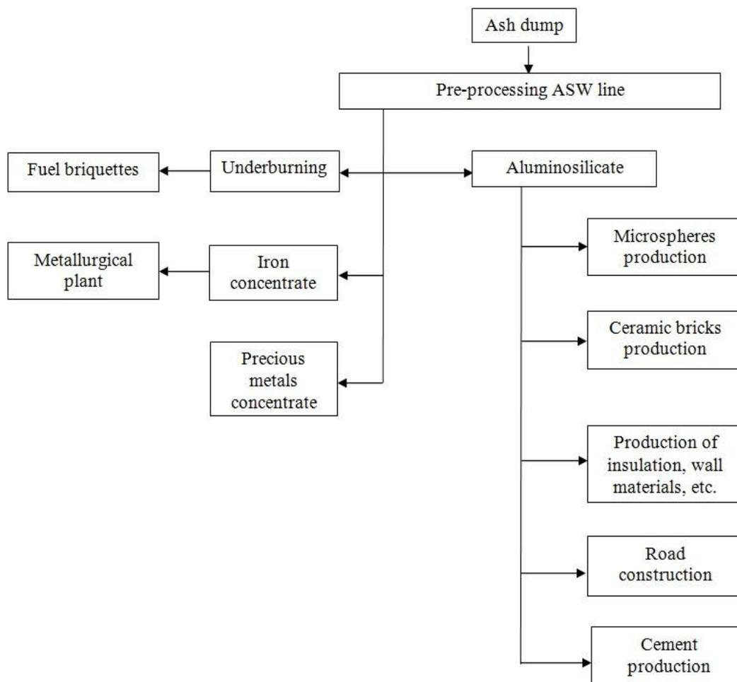
**Fig. 2** - Functional flow diagram of the integrated processing of dump ASW
