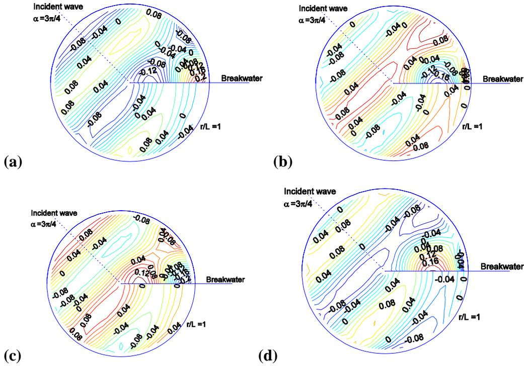
**Figure 3:** Contours of the wave-induced vertical effective normal stresses ( $\sigma'_z / p_0$ ) at  $z=-1$  m for various time intervals. ( $\alpha = 3\pi/4$ ,  $K = 10^{-2}$  m/sec,  $G = 10^7$  N/m<sup>2</sup>). (a)  $t/T=0$ , (b)  $t/T=1/4$ , (c)  $t/T=1/2$  and (d)  $t/T=3/4$ .
