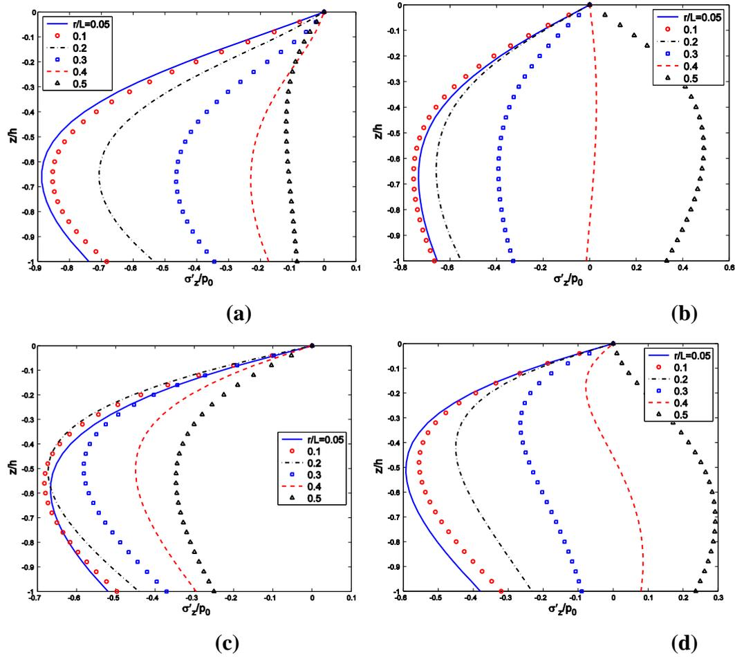
**Figure 7:** Vertical distributions of the wave-induced vertical effective normal stresses ( $\sigma'_z/p_0$ ) for various values of  $r/L$ . ( $K = 10^{-2}$  m/sec,  $G = 10^7$  N/m<sup>2</sup>). (a)  $\alpha = \pi/4$ , (b)  $\alpha = \pi/2$ , (c)  $\alpha = 3\pi/4$  and (d)  $\alpha = \pi$ .
