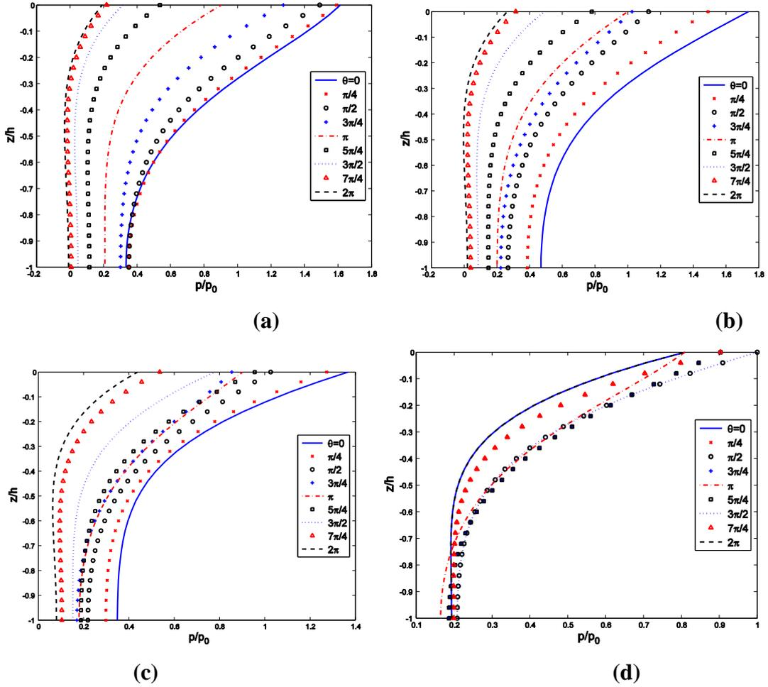
**Figure 4:** Vertical distributions of the wave-induced pore pressure ( $p/p_0$ ) versus  $z/h$  for various values of  $\theta$ . ( $K = 10^{-2}$  m/sec,  $G = 10^7$  N/m<sup>2</sup>). (a)  $\alpha = \pi/4$ , (b)  $\alpha = \pi/2$ , (c)  $\alpha = 3\pi/4$  and (d)  $\alpha = \pi$ .
