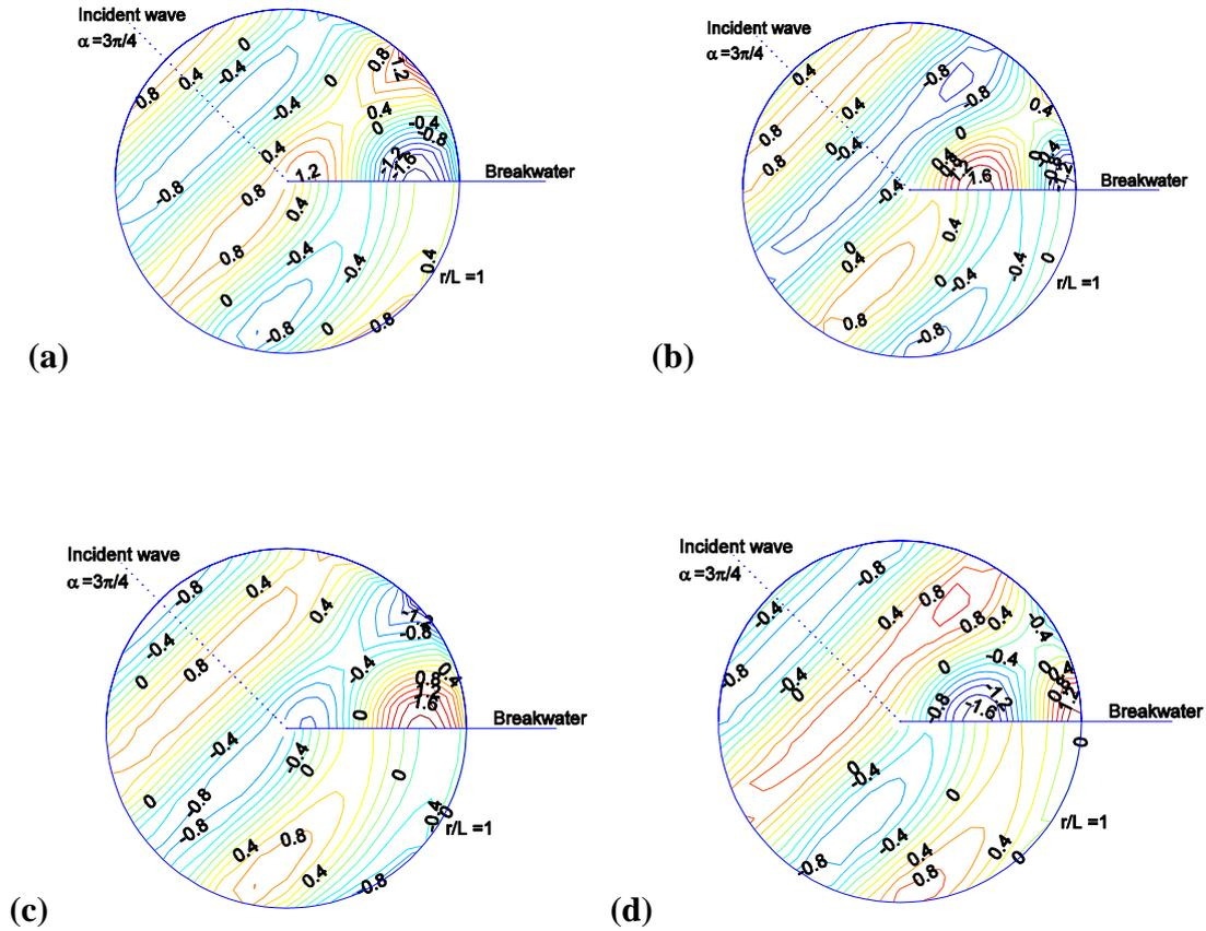
**Figure 2:** Contours of the wave-induced pore pressure ( $p/p_0$ ) at  $z=-1$  m for various time intervals. ( $\alpha = 3\pi/4$ ,  $K = 10^{-2}$  m/sec,  $G = 10^7$  N/m<sup>2</sup>). (a)  $t/T=0$ , (b)  $t/T=1/4$ , (c)  $t/T=1/2$  and (d)  $t/T=3/4$ .
