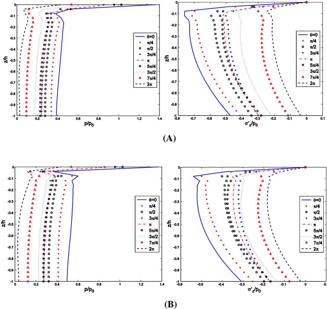
**Figure 8:** Vertical distributions of the wave-induced pore pressure ( $p/p_0$ ) and vertical effective normal stresses ( $\sigma'_z/p_0$ ) versus  $z/h$  for various values of  $\theta$  in different soils. ( $\alpha = 3\pi/4$ ,  $r/L=0.1$ ,  $t=0$ ) (a)  $K = 10^{-4}$  m/sec and  $G = 10^7$  N/m<sup>2</sup> and (b)  $K = 10^{-6}$  m/sec and  $G = 5 \times 10^6$  N/m<sup>2</sup>
