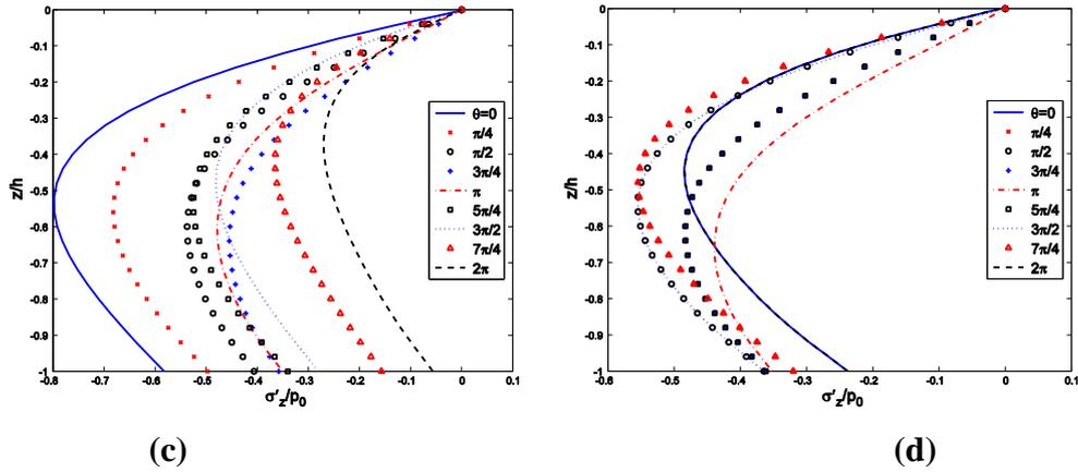
**Figure 5:** Vertical distributions of the wave-induced vertical effective normal stresses ( $\sigma'_z/p_0$ ) for various values of  $\theta$ . ( $K = 10^{-2}$  m/sec,  $G = 10^7$  N/m<sup>2</sup>). (a)  $\alpha = \pi/4$ , (b)  $\alpha = \pi/2$ , (c)  $\alpha = 3\pi/4$  and (d)  $\alpha = \pi$ .
