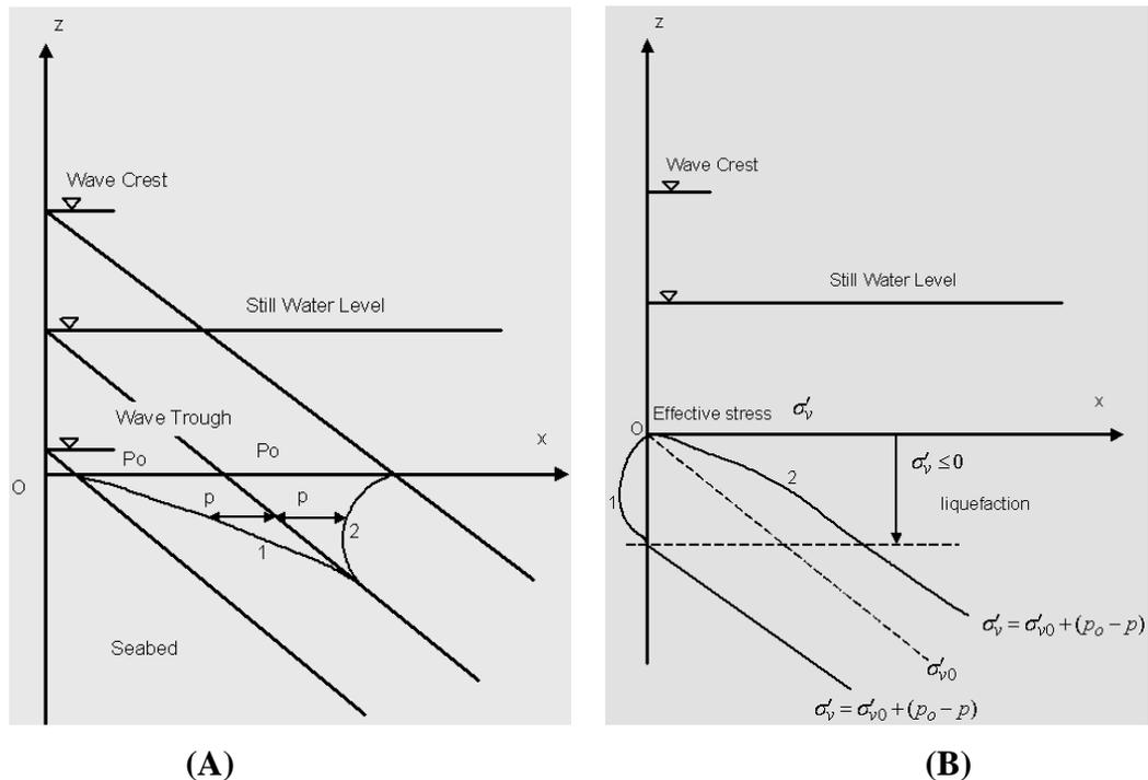
**Figure 9:** Schematic sketch showing definition of liquefaction based on excess pore pressure. (After Zen and Yamamzaki [15]).
