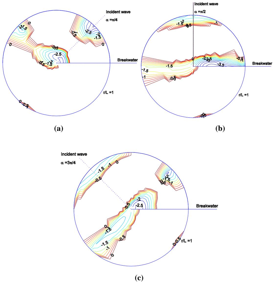
**Figure 10:** The wave-induced liquefaction potential in the vicinity of a breakwater. (a)  $\alpha = \pi/4$ , (b)  $\alpha = \pi/2$  and (c)  $\alpha = 3\pi/4$ . ( $K = 10^{-4}$  m/sec,  $G = 10^7$  N/m<sup>2</sup>) (a)  $\alpha = \pi/4$ , (b)  $\alpha = \pi/2$  and (c)  $\alpha = 3\pi/4$ .
