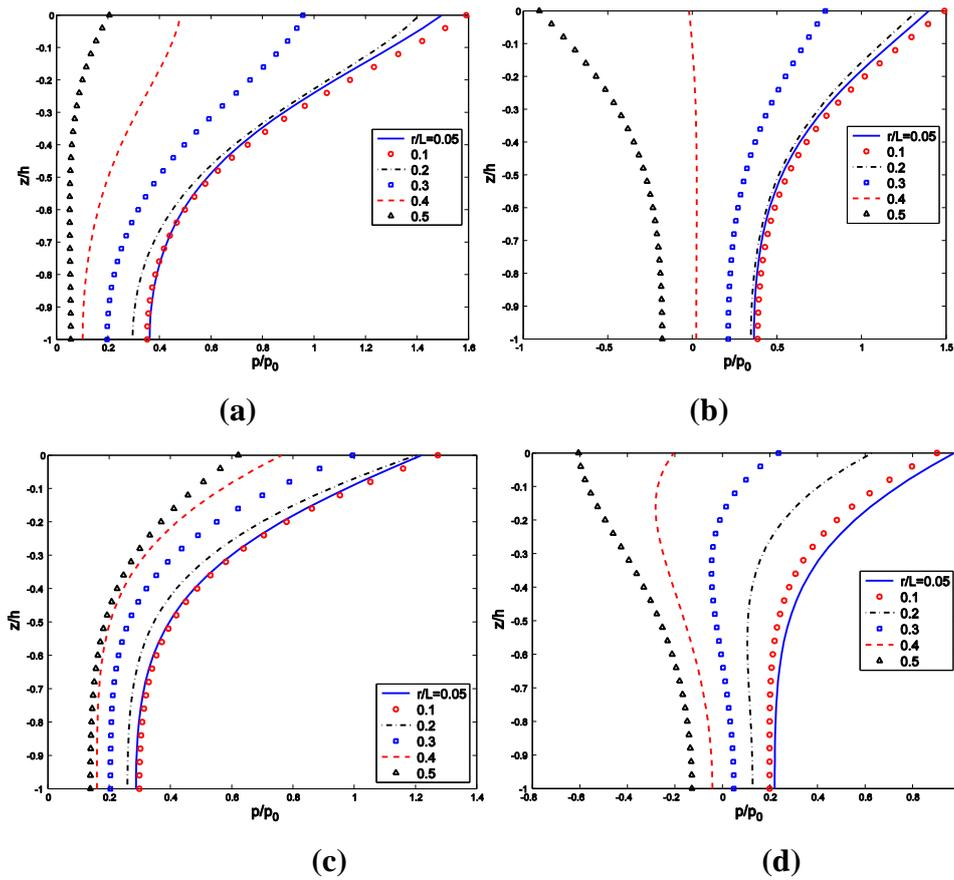
**Figure 6:** Vertical distributions of the wave-induced pore pressure ( $p/p_0$ ) versus  $z/h$  for various values of  $r/L$ . ( $K = 10^{-2}$  m/sec,  $G = 10^7$  N/m<sup>2</sup>). (a)  $\alpha = \pi/4$ , (b)  $\alpha = \pi/2$ , (c)  $\alpha = 3\pi/4$  and (d)  $\alpha = \pi$
