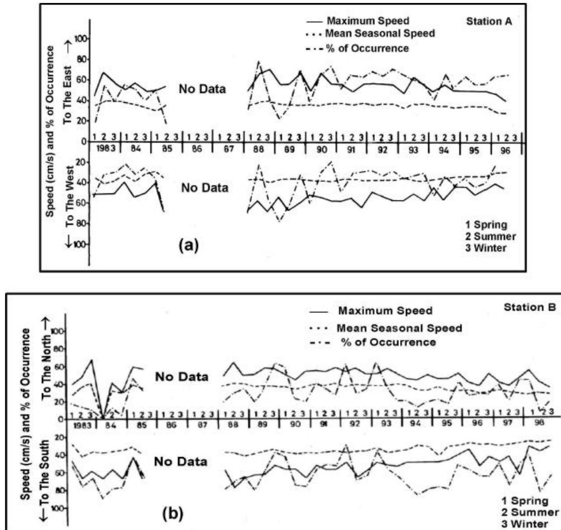
**Figure 2.** Long-term (seasonal and annual) mean cumulative frequency curves of long-shore currents: a- at station A east of Rosetta estuary during 1983-1996 and b- at station B westward of Rosetta mouth during 1983-1998.
