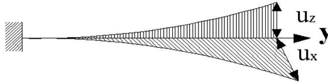
**Figure 2.**Deformation of the beam in x-y and y-z plane [7]
