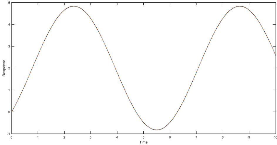
**Figure 3.**Response versus time for unit velocity as initial condition
