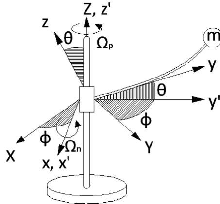
**Figure 1.**Motion of the beam about a point (spin is not shown in the figure to avoid complexity) [7]
