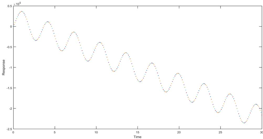
**Figure 4.**Response versus time for unit displacement as initial condition
