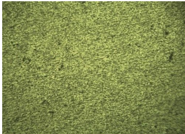
Fig.6 (a) Microstructure of parent metal
