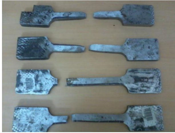
Fig. 2 Specimens for UTS test
