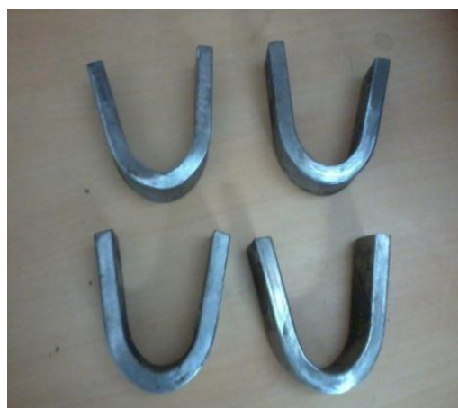
Fig 5. Specimens after bend test
