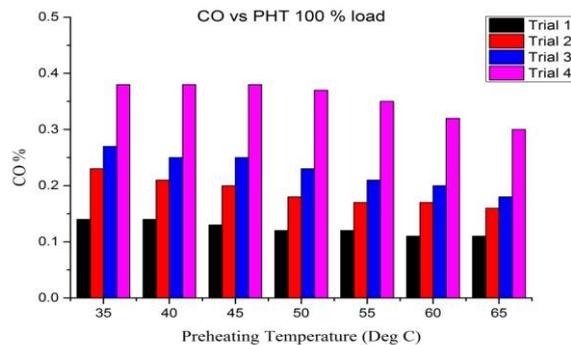
**Fig. 5** Carbon monoxide V/s Preheating Temperature for different vapor induction at 100 % load
