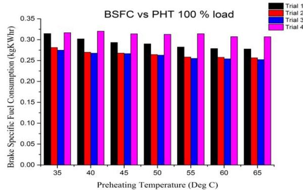
**Fig 3.** Brake Specific Fuel Consumption V/s Preheating temperature for different vapor induction at 100 % load
