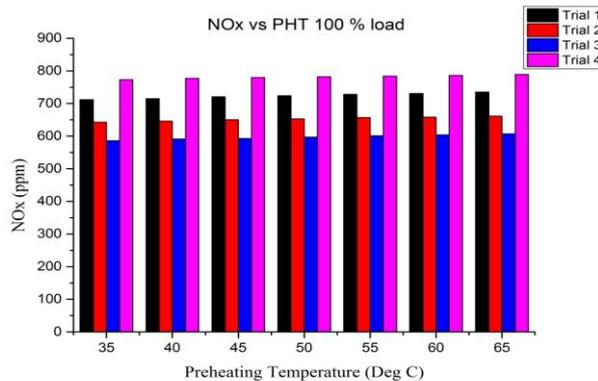
**Fig 6.** NO<sub>x</sub> vs Preheating temperature for 100 % load at different vapor induction
