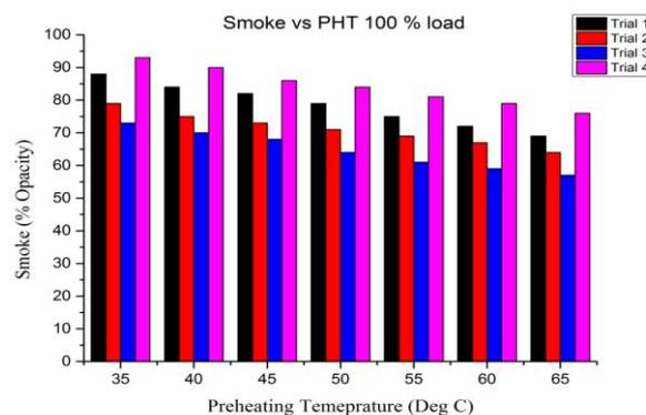
**Fig 7.** Smoke opacity V/s Preheating temperature for 100 % load for different vapor induction
