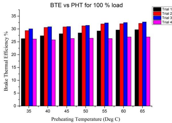
**Fig 2.** Brake thermal Efficiency V/s Preheating temperature for different vapor induction at 100 % load
