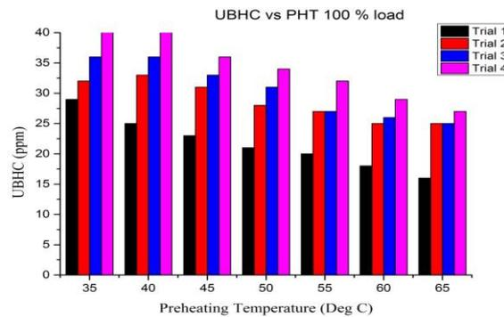
**Fig 4.** Unburned Hydrocarbons vs Preheating Temperature for different vapor induction for 100 % load
