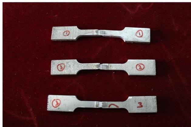
**Fig. 7.** Tensile Specimens after Tensile Test
