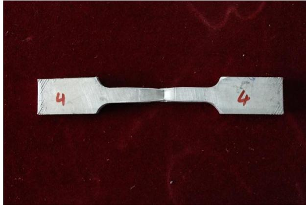
**Fig. 8.** Tensile Specimens after Tensile Test
