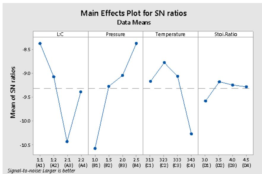
Fig .3. Mean S/N ratio plot for L:C (A1-A4),Pressure (B1-B4),Temperature (C1-C4), Stoi.Ratio (D1-D4)
