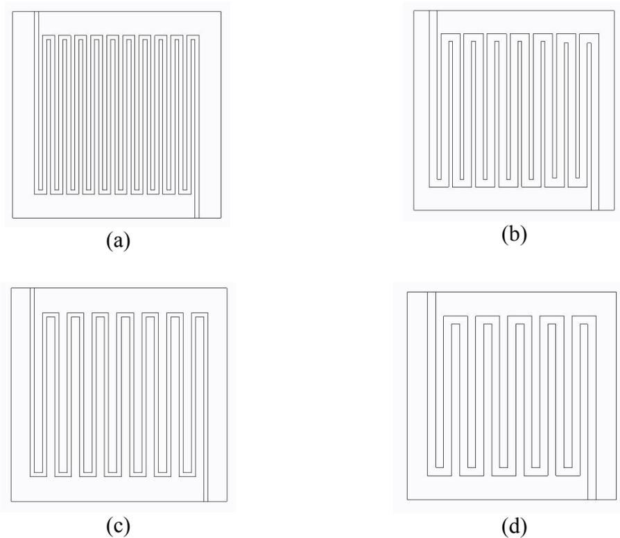
**Fig.1.** Various landing to channel width (L: C) (a) 1:1 (b) 1:2 (c) 2:1 and (d) 2:2 of serpentine flow channel of 16 cm<sup>2</sup> active area of PEMFC
