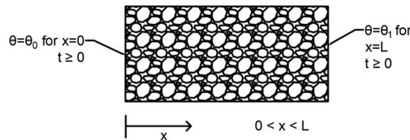
**Figure 1** One Dimensional Horizontal Column
