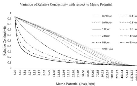
**Figure 5** Variation of Relative conductivity with respect to Matric Potential
