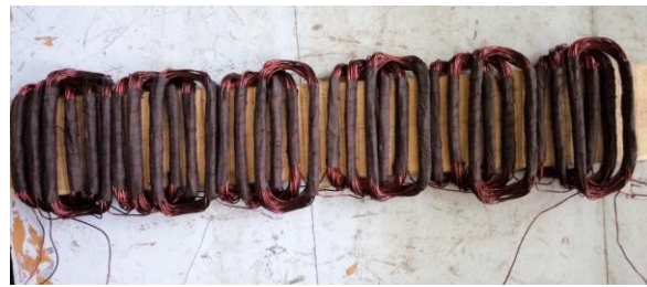
Fig. 14 Removed wooden strips and coils are taped with insulation
