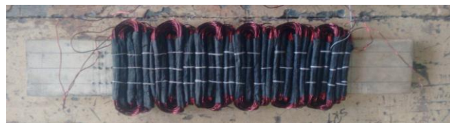
Fig. 15 Coils of three phases, taped, hammered and held together by thread
