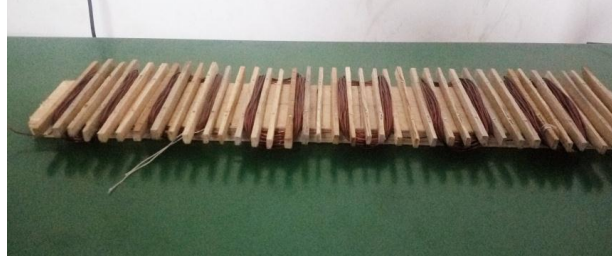
Fig. 13 One phase windings around wooden strips
