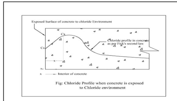
**Figure.3:** Chloride Profile when concrete in exposed to chloride environment
