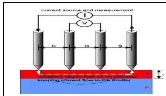
**Figure.6:** Arrangement of Electrical Resistivity Method
