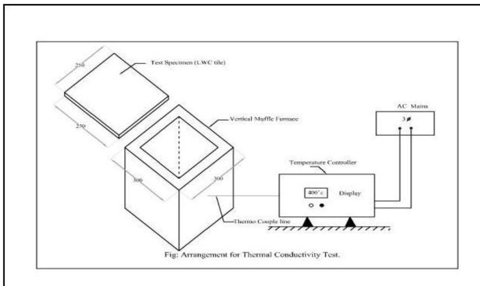
**Figure 9:** Arrangement for thermal conductivity test
