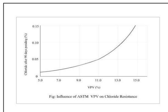
**Figure 5:** Influence of ASTM VPV on chloride resistance
