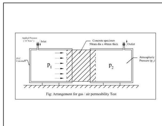
**Figure 7:** Arrangement of Air/gas Permeability Test Intrinsic gas permeability
