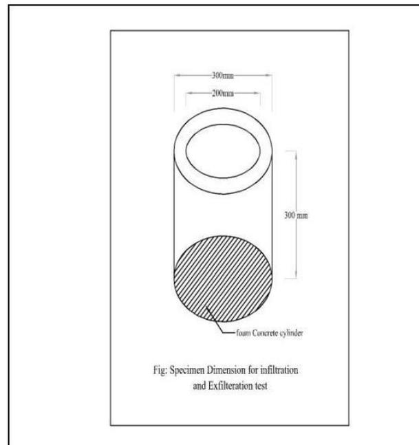
**Figure 11:** Specimen dimension for Infiltration and Exfiltration
