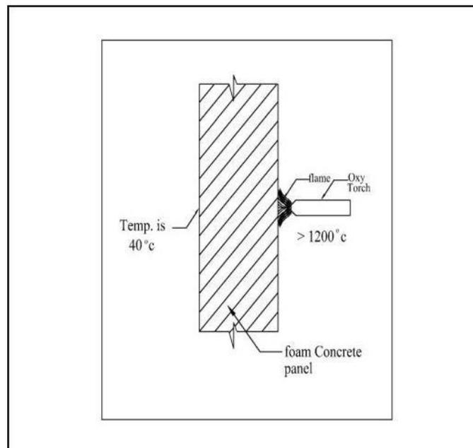
**Figure 10:** Arrangement of Flame resistance test
