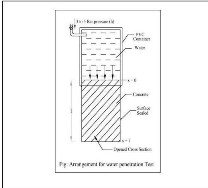
**Figure 8:** Arrangement for water penetration test
