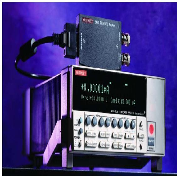
Figure 4. Electrometer
