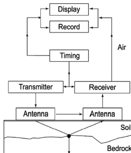
**Figure1.** Ground Penetration Radar (GPR) system
