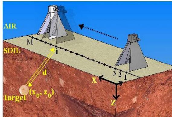
**Figure 2.** Stepped Frequency GPR
