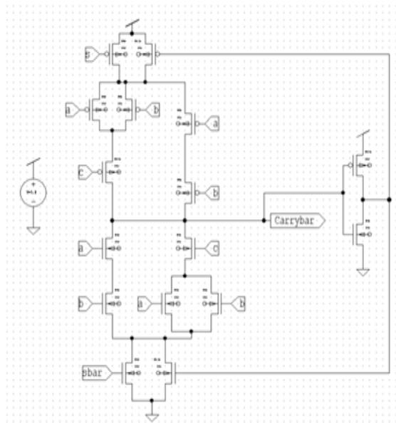
Fig.10 Inverted carry logic using Leakage Feedback approach
