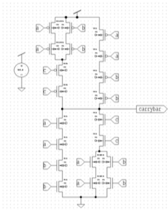
Fig.4 inverted carry logic using stack approach
