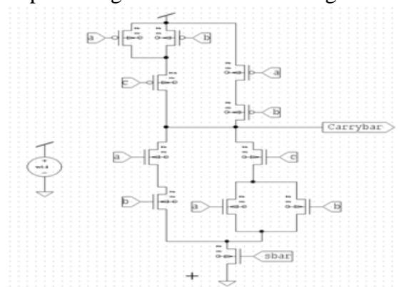
Fig.8 Inverted carry logic using zigzag approach
