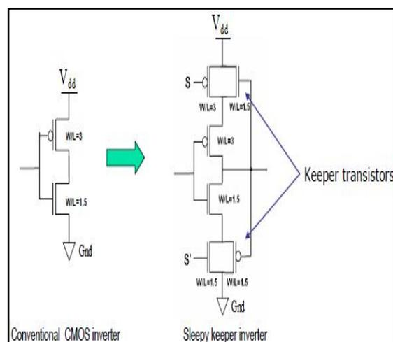
Fig12. Sleepy keeper for CMOS inverter
