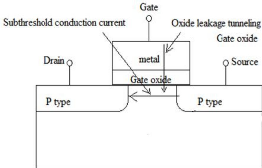
Figure.1 Different types of leakage currents in MOSFET
