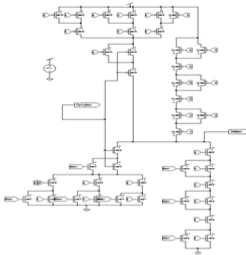
Fig.6 Inverted carry logic using sleepy stack approach
