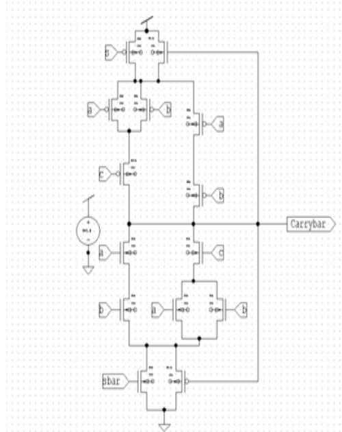
Fig.13. Inverted carry logic using sleepy keeper approach
