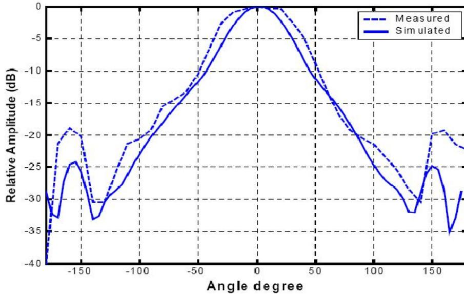
**Figure 5:** Measured and simulated H-plane field with horn.
