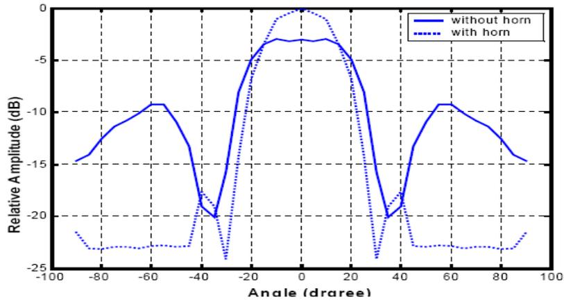
Figure 7: Two-Element measured E-plane field with and without horn.
