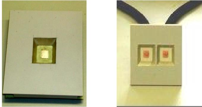
**Figure 3:** Fabricated Patch with Surface Mount Quasi-Planar.
