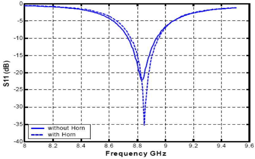
Figure 6: Measurement of return-loss with and without horn.
