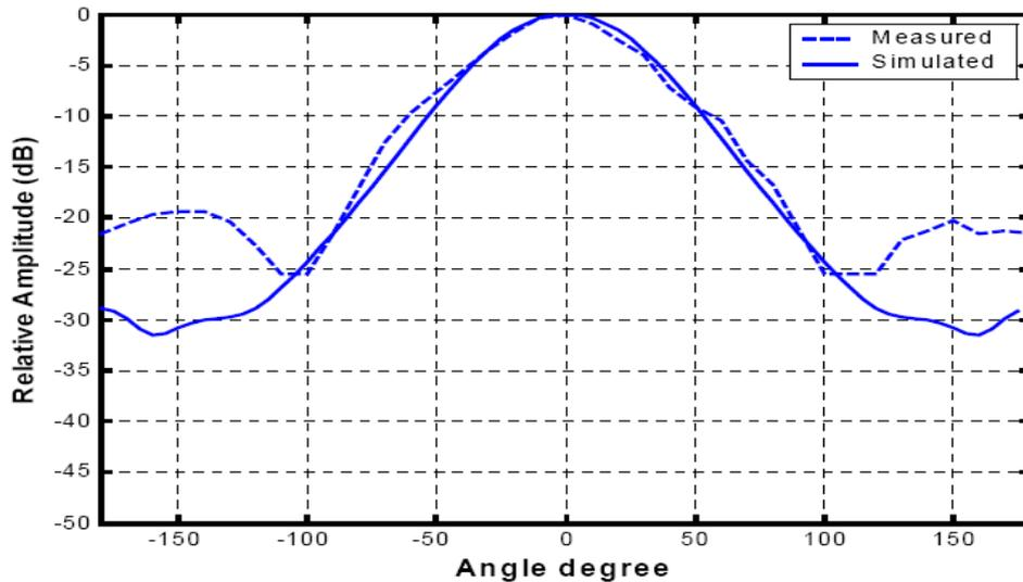
**Figure 4:** Measured and simulated E-plane field with horn.
