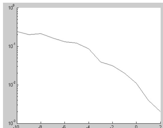
**Fig. IV:** BER performance in a downlink CDMA system in an AWGN channel.
