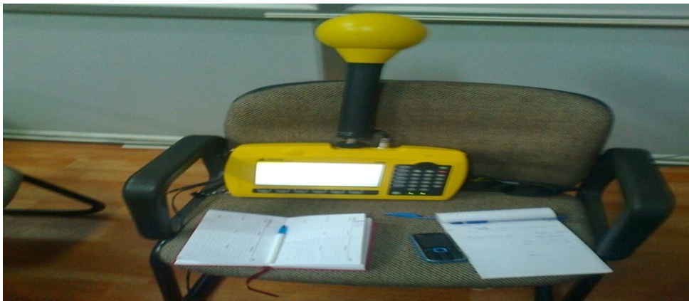
Fig. 1: Selective Radiation Meter SRM-3006.
