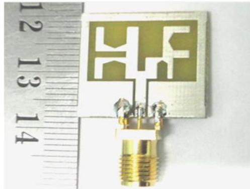
**Figure 2:** Fabricated bevel U-L shaped antenna
