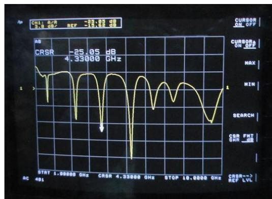
**Figure 6:** Measurement of Return Loss At 4.3GHz
