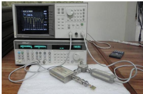
**Figure 5:** Return loss measurement using HP 8757D Scalar NW Analyzer for a bevel U-L shaped antenna
