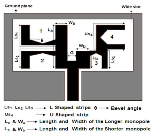
**Figure 3:** Parameters of bevel U-L shaped antenna
