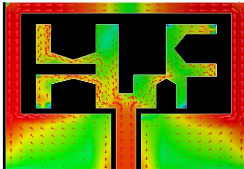
**Figure 6(b):** Surface Current Distribution at 7.4GHz
