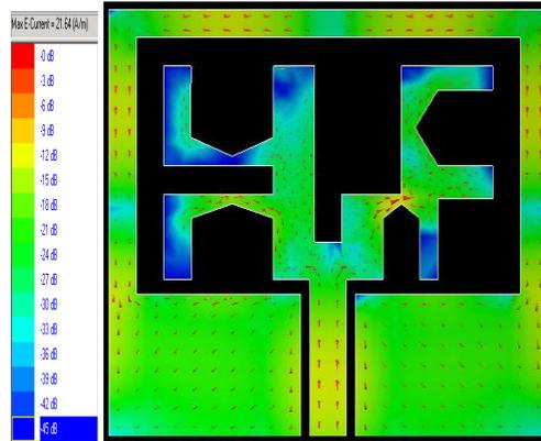
**Figure 6(a):** Surface Current Distribution at 4.3GHz
