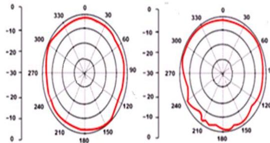
**Figure 7 (b):** Radiation pattern at 4.3 GHz and 7.4 GHz H-plane (XY)
