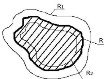
**Fig. 2.** Shadow boundary, inner and outer outline lines
