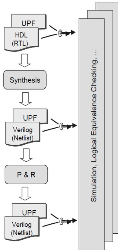
FIG 2: UPF VALIDATION AT DIFFERENT DESIGN STAGES
