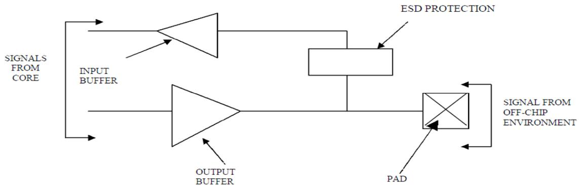
FIG 1: BLOCK DIAGRAM OF BIDIRECTIONAL BUFFER
